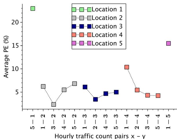
Fig. 4 The average PE of the pointer prediction of the 14 traffic count pairs *x-y*.
