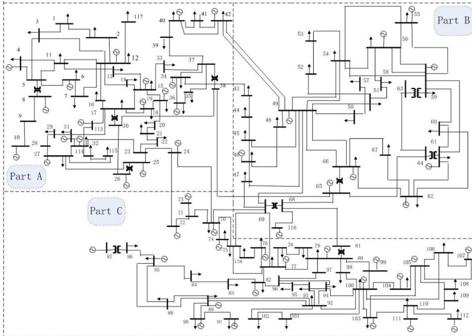
Fig. 3 Network simplification of IEEE standard 118-bus system.
