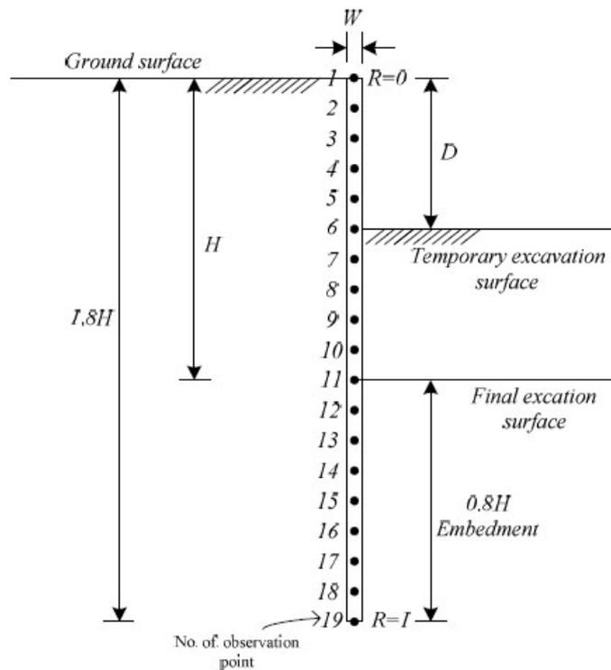
Fig. 4 Representation of the diaphragm wall structure system [12].
