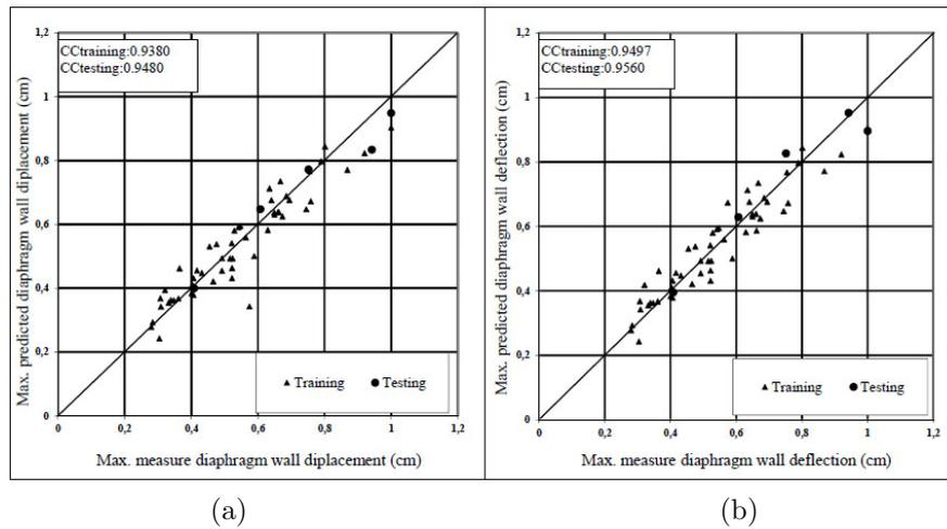
**Fig. 5** Measured vs. predicted maximum diaphragm wall deflection: (a) with linear time function; (b) with quadratic time function.
